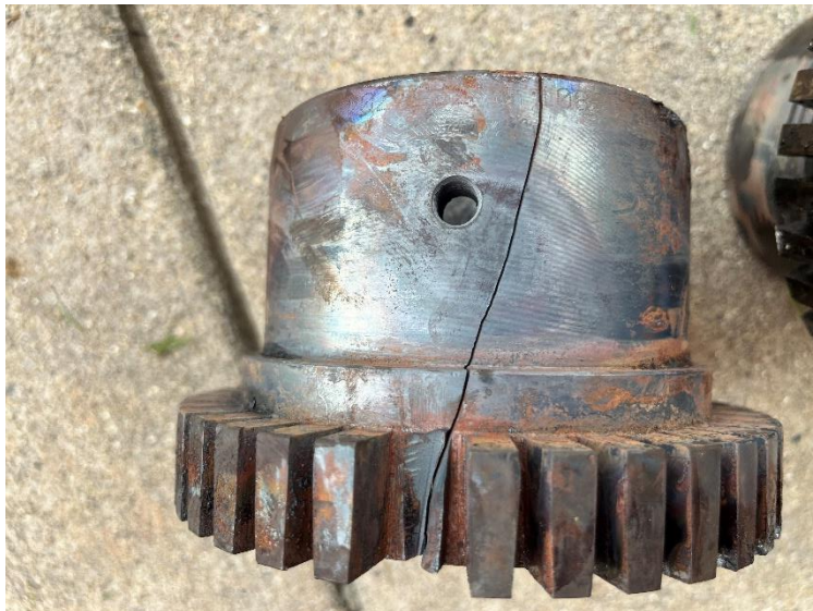
Blower Coupling Failure Picture
