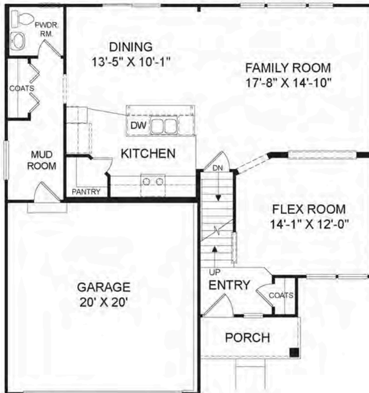
FIRST FLOOR 8' CEILING HT. DIMENSIONS 38'W x 40'D 2008 SF TOTAL
