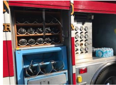
air fill containment system
